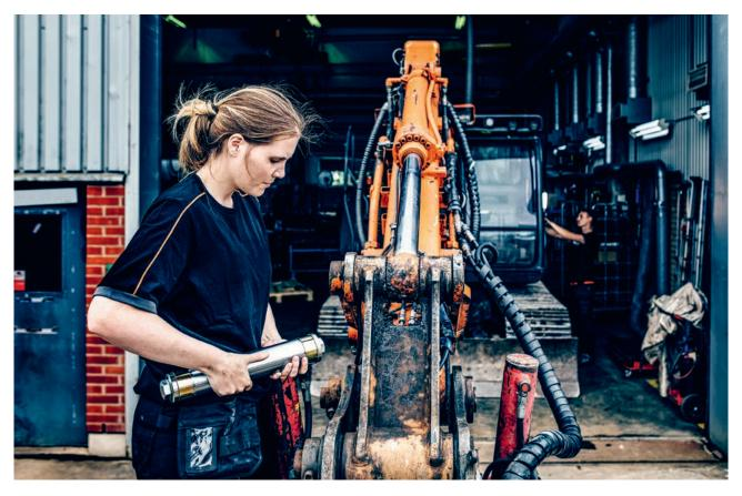
Expander System is an award-winning pivot pin solution with more than one million systems installed since 1985. The design can be adapted to each individual application, for example offering a permanent repair method for joint lug wear in heavy machinery equipment.
