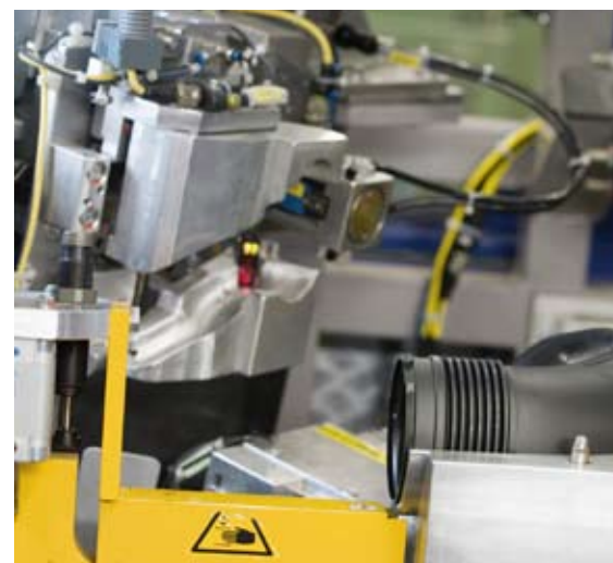
High level of mechanised production. This shows the finishing dressing of a blow moulded air intake pipe.
