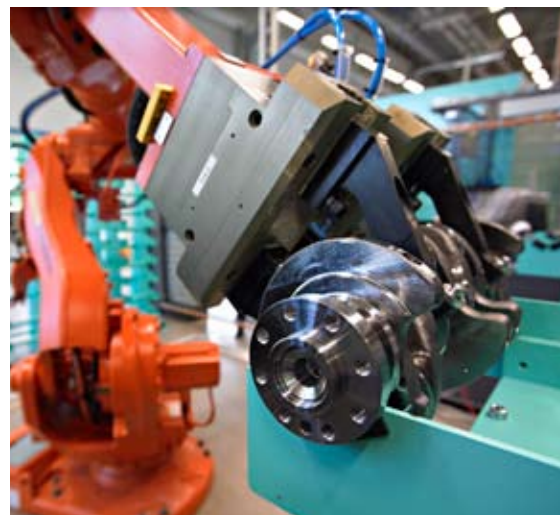
Work on a crankshaft with the help of a robot.
