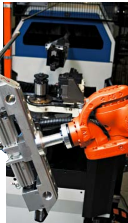
Automated production cells for bending, endforming, brazing and washing AC pipes.
