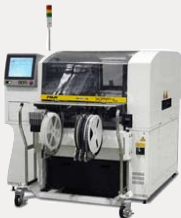
Fuji XPF mounting machine for circuit card production.
