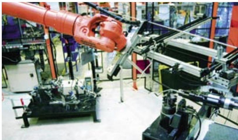
Robotic bending of fuel lines as well as leak testing.
