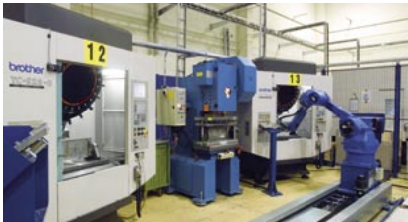
This is a typical interior in a modern Swedish engineering company – clean, efficient and unmanned. Hellmer Industrier in Norrköping has 16 machines from Japanese Brother delivered by Mekana for the manufacture of details to the telecom industry.
