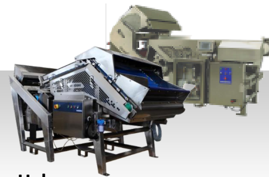
New Halo High Resolution Sort For whole fruits and vegetables – Color, Defect, Size, Shape & Safety
